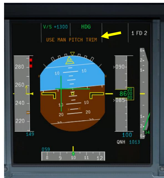
TEST 2: ELAC 1 and ELAC 2 off and landing gear deployed = DIRECT LAW
