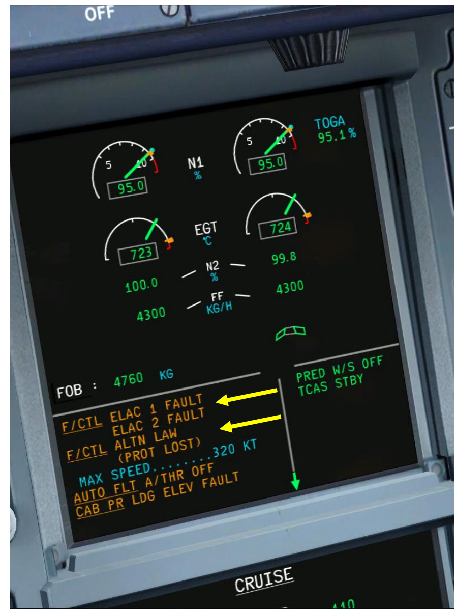
TEST 1: ELAC 1 and ELAC 2 off = ALTERNATE LAW
